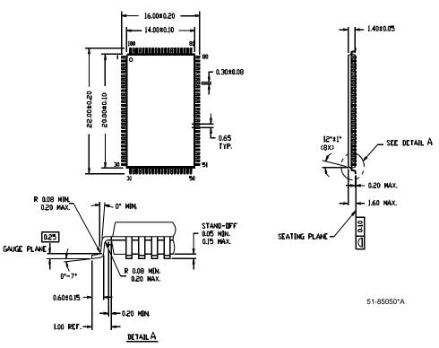
DIMENSIONS ARE IN MILLIMETERS.
