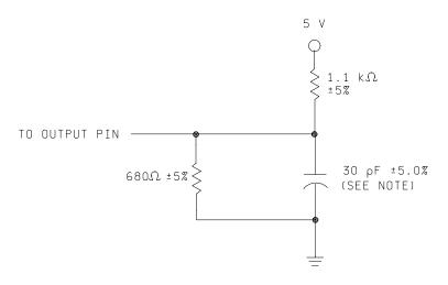
NOTE:  $C_L$  includes scope and jig capacitance.
