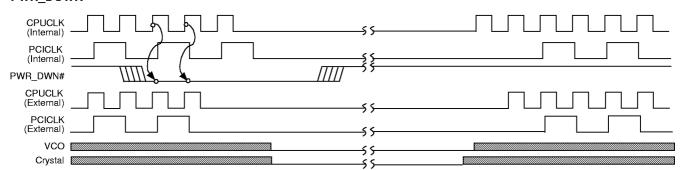
Shaded section on the VCO and Crystal waveforms indicates that the VCO and crystal oscillator are active, and there is a valid clock.
