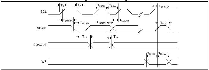
Figure 5-12. Write Cycle Timing
