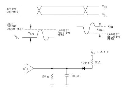
NOTE: Resistor and capacitor tolerances =  $\pm 10\%$
