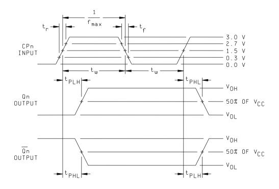
FIGURE 5. Switching waveforms and test circuit.
