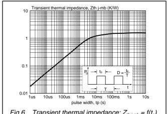
Fig.6. Transient thermal impedance;  $Z_{th j-mb} = f(t_p)$ .
