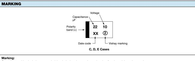
Capacitor marking includes an anode (+) polarity band, capacitance in microfarads and the voltage rating.
