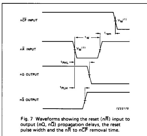
Fig. 7 Waveforms showing the reset ( $nR$ ) input to output ( $nQ$ ,  $n\bar{Q}$ ) propagation delays, the reset pulse width and the  $nR$  to  $nCP$  removal time.
