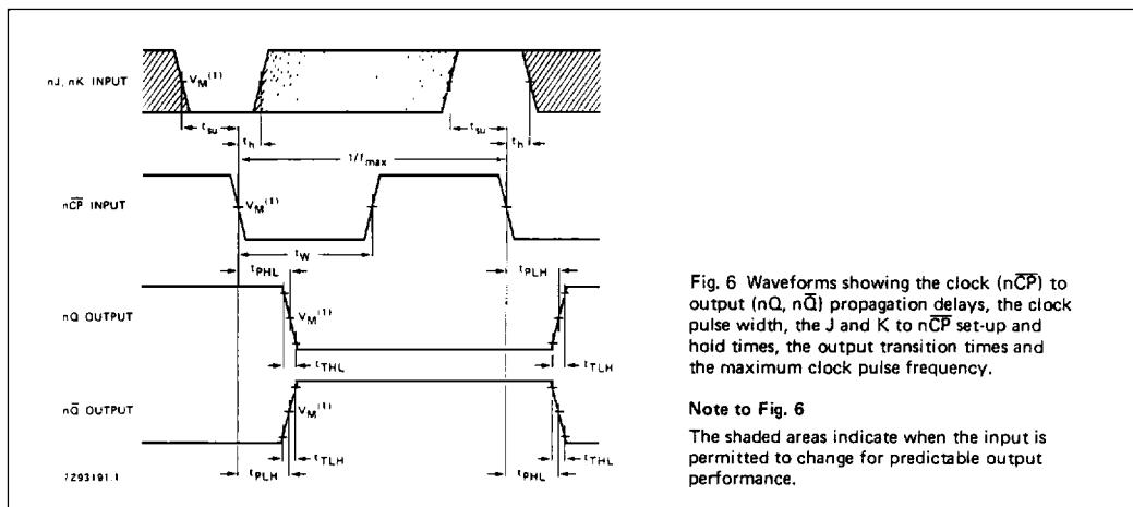
Fig. 6 Waveforms showing the clock ( $nCP$ ) to output ( $nQ$ ,  $n\bar{Q}$ ) propagation delays, the clock pulse width, the  $J$  and  $K$  to  $nCP$  set-up and hold times, the output transition times and the maximum clock pulse frequency.
