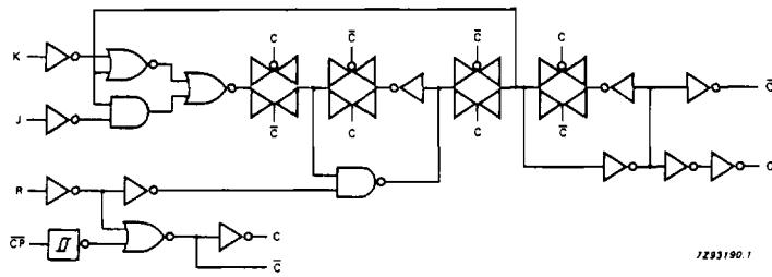
Fig. 5 Logic diagram (one flip-flop).
