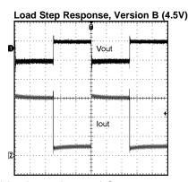
$V_{IN}$  = 3.6V, Load = 20mA - 150mA Step CH1 (top):  $V_{OUT}$ ; Scale: 50mV/Div, AC Coupled
