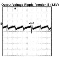
$V_{IN} = 3.6V$ , Load = 150mA
