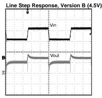
$$\begin{split} &V_{\text{IN}} = 3.2 \text{V} - 4.2 \text{V Step, Load} = 150 \text{mA} \\ &\text{CH1 (top): } &V_{\text{IN}}; \text{ Scale: } 1 \text{V/Div, DC Coupled} \\ &\text{CH2: } &V_{\text{OUT}}; \text{ Scale: } 50 \text{mV/Div, AC Coupled} \end{split}$$
