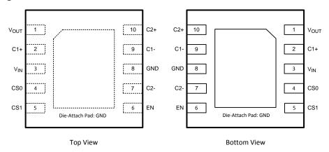
Figure 1. 10-pin SON No Pullback Package (3mm × 3mm × 0.8mm) See Package Number DSC0010A
