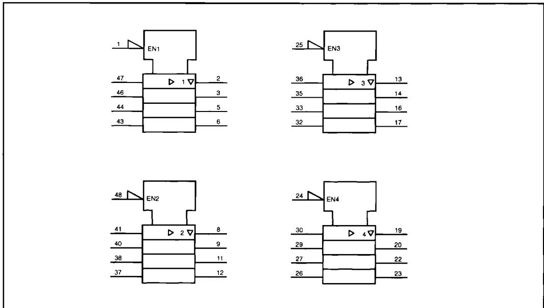
**3.3V ABT 16-Bit buffers/drivers with 30Ω termination
