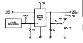
Note: C<sub>4</sub> includes test fixture capacitance. Port input is in a fixed logical condition.
