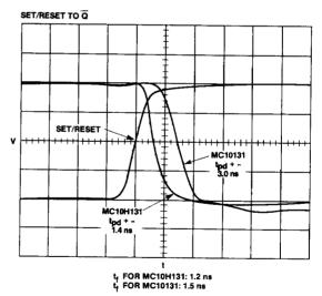
NOTE:  $t_f$  and  $t_f$  measured from the 20% to the 80% level of the output signal swing.  $t_{pd}$  is measured from the 50% level of the input to the 50% level of the output.
