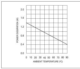
Figure 7. Maximum Power dissipation (SOT89)
