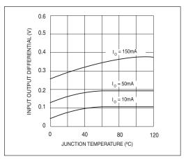
Figure 3. Dropout Voltage
