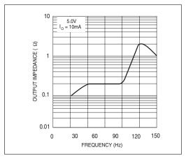
Figure 9. Output Impedance
