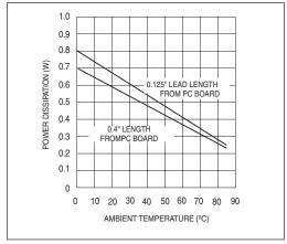
Figure 8. Maximum Power Dissipation (TO-92)
