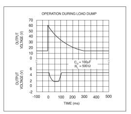
Figure 10. Operation During Load Dump
