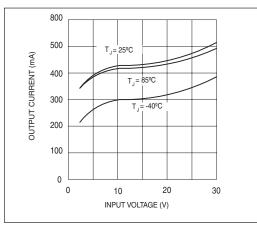
Figure 5. Peak Output Current
