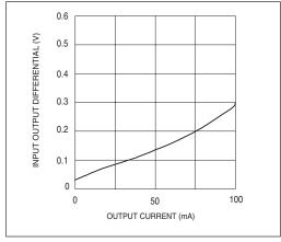
Figure 4. Dropout Voltage
