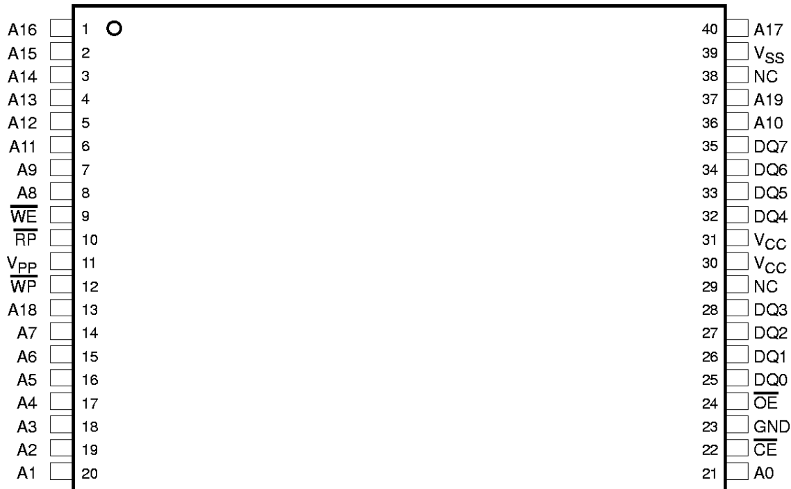
TMS28F008Axy 40-PIN TSOP (DCD) (TOP VIEW)
