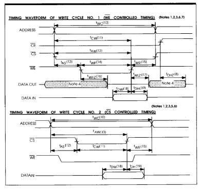
Writing to the S128K8 is achieved when the chip select (CS) and write enable (WE) inputs are LOW. Data on the input/output pins is written into the memory location specified on the address pins (A0-A16).
