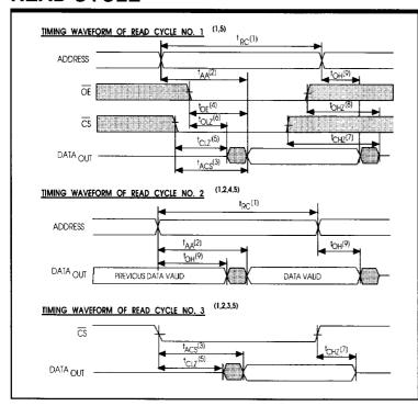
Reading the S128K8 device is accomplished by taking chipselect (CS) and output enable (OE) LOW, while write enable (WE) remains inactive or high. Under these conditions, the contents of the memory location specified on the address pins will appear on the appropriate data input/output pins.
