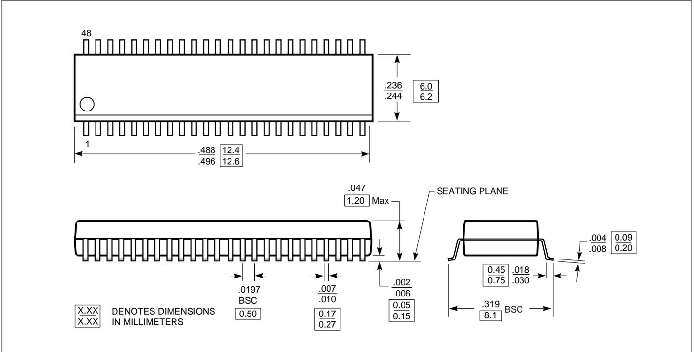
**Packaging Mechanical: 48-pin 300 mil wide plastic SSOP (V)**
