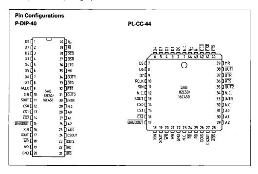
The SAB 82C50/16C450 (UART) performs serial-to-parallel conversion on data characters received from a peripheral device or a modem, and parallel-to-serial conversion on data characters received from the CPU. The CPU can read the complete status of the UART at any time during the functional operation. Status information reported includes the type and condition of the transfer operations being performed by the UART, as well as any error condition (parity, overrun, framing, or break interrupt).
