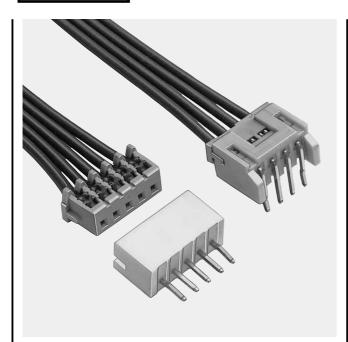
The CR 2.0mm (.079") insulation displacement connector features a mounting height as low as 6.9mm (.272") and a thickness as thin as 4.8mm (.189") (for top entry type). It's suitable for interconnection of UL1007 electric wires in a wide range of electrical and electronic equipment such as VCRs and video cameras.
