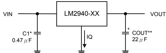
\*Required if regulator is located far from power supply filter.
