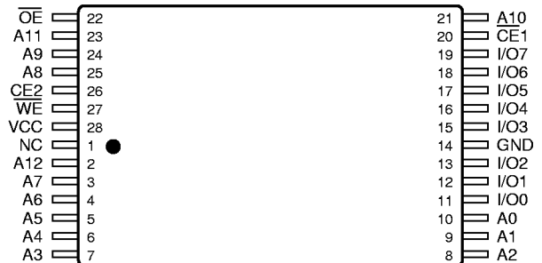
28-Pin TSOP (Standard)
