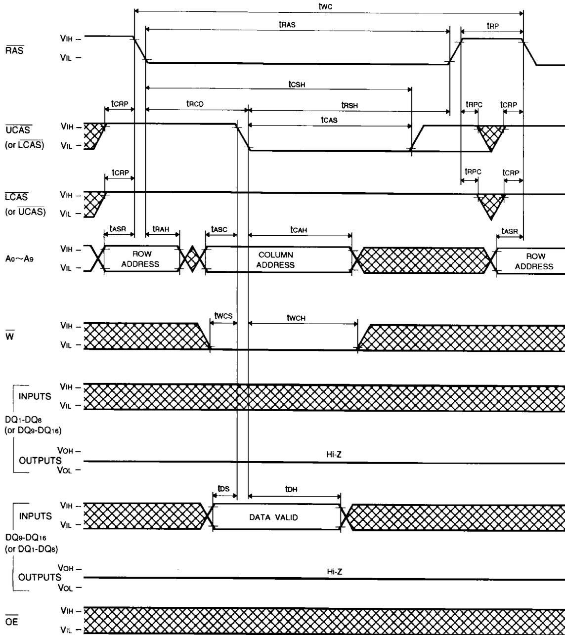
**Upper / (Lower) Byte Write Cycle (Delayed write)**
