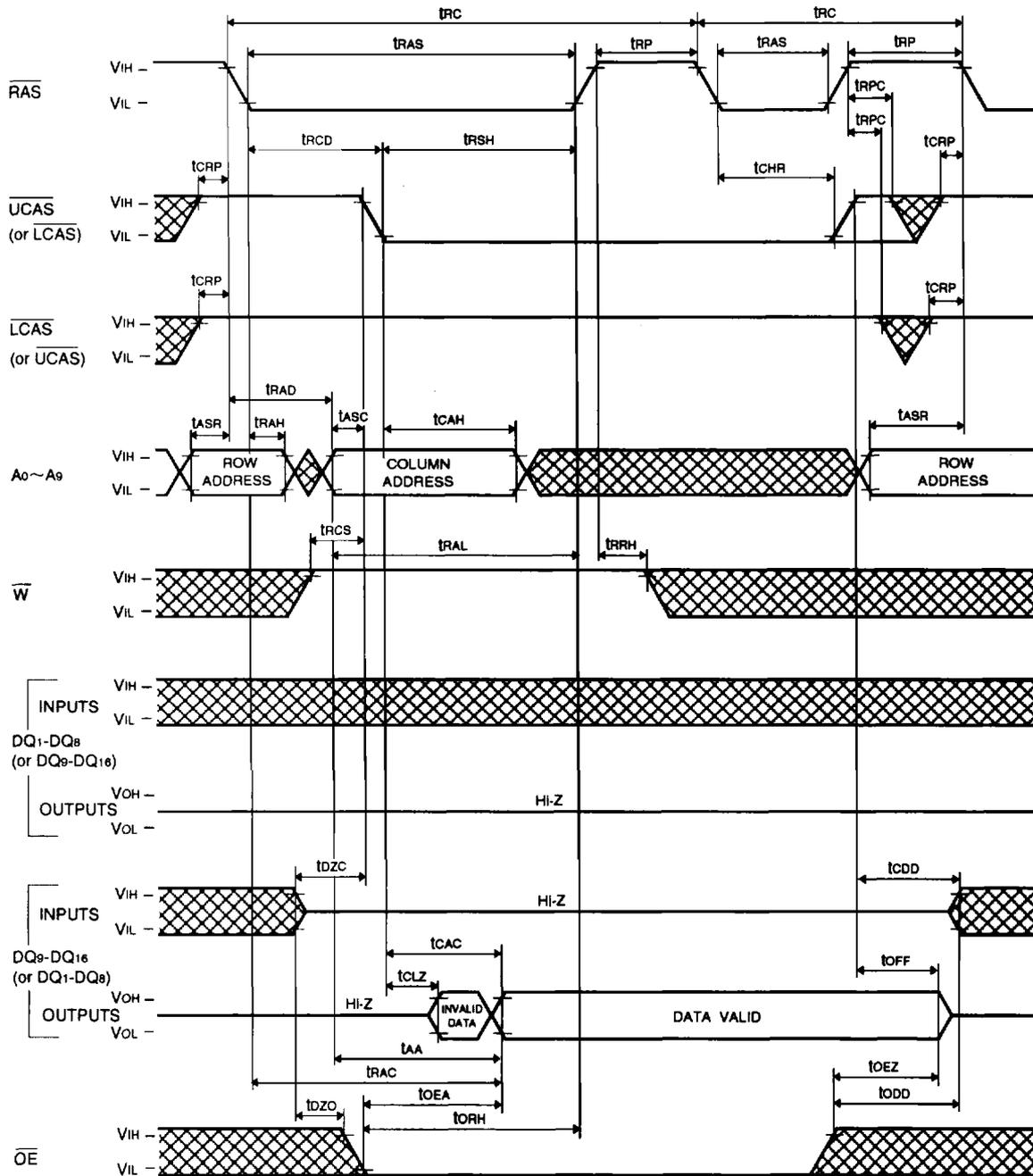
Note 29: Early write, delayed write, read write or read modify write cycle is applicable instead of read cycle. Timing requirements and output state are the same as that of each cycle shown above.
