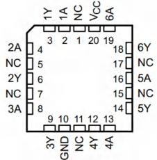
Figure 4-1. SN54AHC04 J or W Package SN74AHC04 D, DB, DGV, N, NS, or PW Package (Top View)
