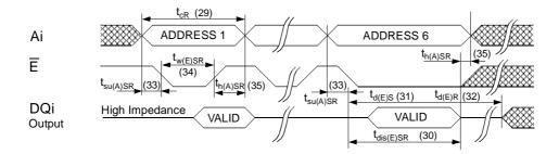
u:  $\overline{W}$  must be HIGH when  $\overline{E}$  is LOW during the address sequence in order to initiate a nonvolatile cycle.  $\overline{G}$  may be either HIGH or LOW throughout. Addresses 1 through 6 are found in the mode selection table. Address 6 determines wheter the UL635H256 performs a STORE or RECALL.
