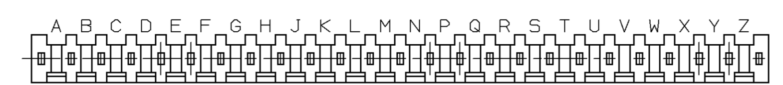
KEYWAY LOCATIONS (REF-SEE TABLE) (MATING LENGTH OF POST ON NEAR SIDE) SCALE: 2:1
