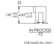
NOTE: DIMENSION APPLIES PRIOR TO RE-PRESS, SEE SECTION "B-B" FOR FINISHED DIMENSION
