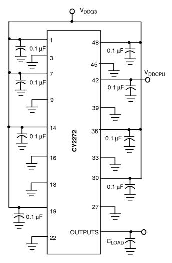
Note: All Capacitors must be placed as close to the pins as is possible
