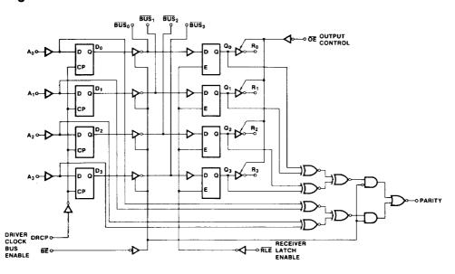
data regardless of the bus input. The four latches have threestate outputs and are controlled by a buffered common threestate control (OE) input. When OE is HIGH, the receiver outputs are in the high-impedance state.
