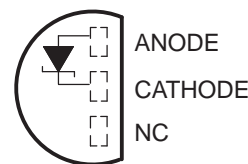
LP (TO-92/TO-226) PACKAGE (TOP VIEW)
