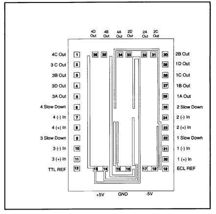
Slow down pads are for use when switching speeds are not critical but in band RF noise is. Capacitor installed from slow down pad to -Vee or ground.
