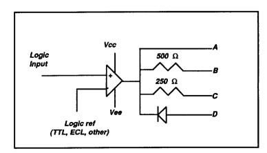
With the (-) input tied to the desired logic, the driver will be non-inverting, with the (+) input tied to desired logic driver will be inverting.
