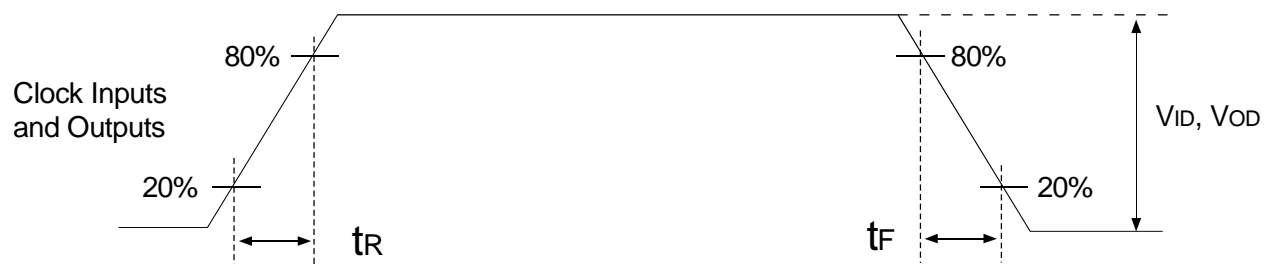
Figure 8. Input and Output Slew Rates
