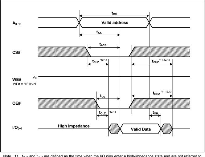
Note 11.  $t_{CHZ}$  and  $t_{OHZ}$  are defined as the time when the I/O pins enter a high-impedance state and are not referred to the I/O levels.
