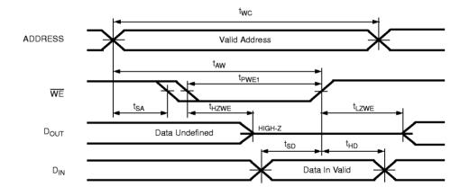
Write Cycle No.3 (WE controlled, OE is LOW, CE is LOW: WE Terminates Write) 10
