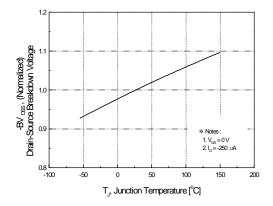
Figure 7. Breakdown Voltage Variation vs. Temperature
