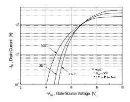
Figure 2. Transfer Characteristics
