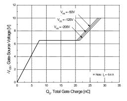
Figure 6. Gate Charge Characteristics
