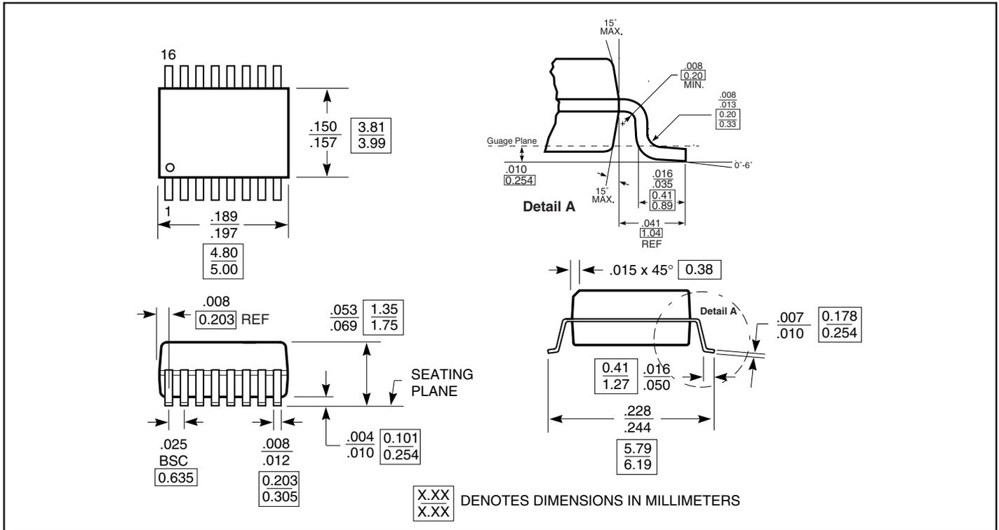
**Packaging Mechanical: 16-pin SOIC (W)**
