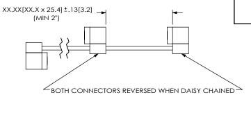
FIG 5 (FFSD-10-D-XX.XX-01-X-N-DXX-M SHOWN) (SAME AS FIG 1, DIFFERENT AS SHOWN) (2.00[50.8] MINIMUM, 1.00[25.4] INCREMENTS)
