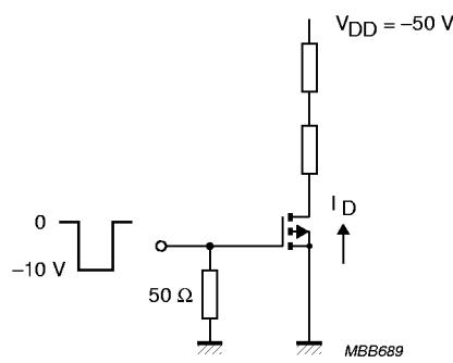
Fig.2 Switching time test circuit.
