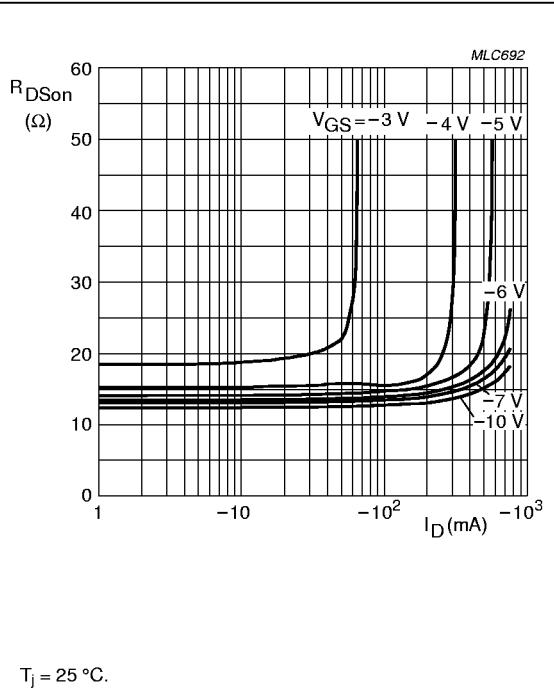
Fig.10 Drain-source on-state resistance as a function of drain current; typical values.
