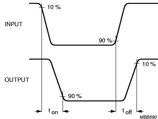
Fig.3 Input and output waveforms.
