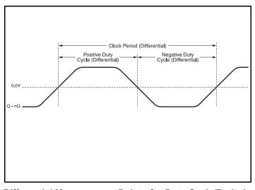
**Differential Measurement Points for Duty Cycle/Period**
