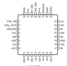
841608 32-Lead VFQFPN 5mm x 5mm x 0.925mm package body K Package Top View
