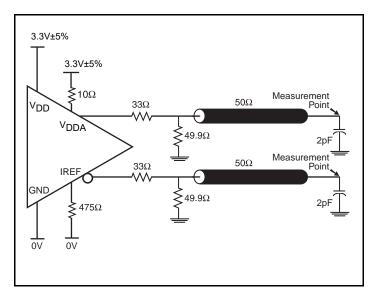
3.3V HCSL Output Load AC Test Circuit
