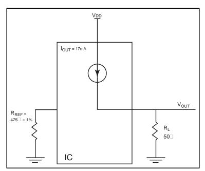
Figure 7. HCSL Driver Circuit and Termination
