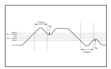
**Differential Measurement Points for Ringback**
