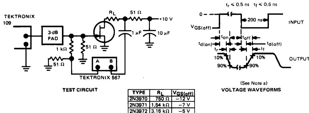
**NOTE a:** An equivalent generator and oscilloscope may be used. The oscilloscope must have a  $50\text{-}\Omega$  input impedance.
