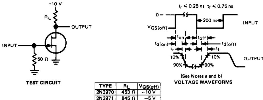
**NOTES:** a. The input waveforms are supplied by a generator with the following characteristics:  $Z_{out} = 50\ \Omega$ , duty cycle  $\approx 2\%$ .
