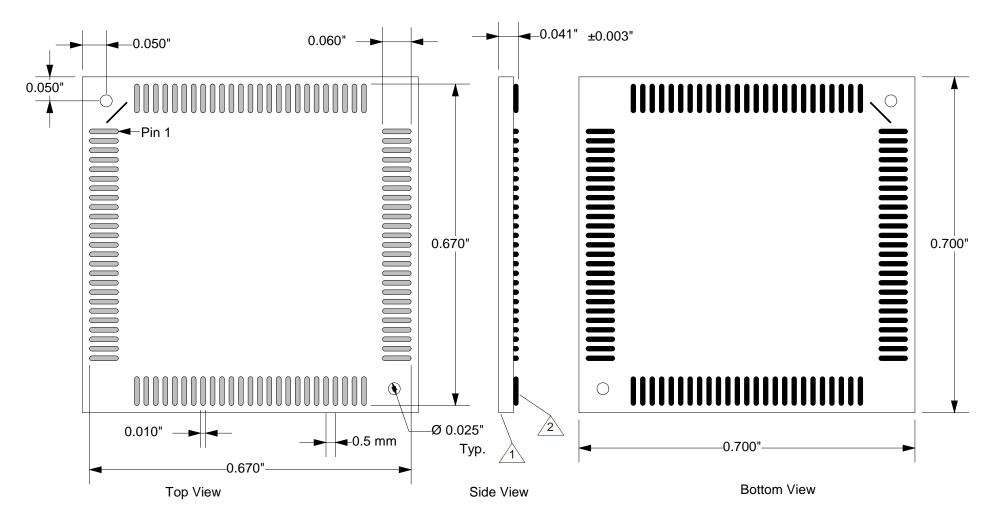
Substrate: 0.0315"±0.007" FR4/G10 or equivalent high temp material.
