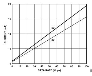
Figure 9. Typical ADuM2280 or ADuM2285 V<sub>DD1</sub> Supply Current vs. Data Rate for 5 V and 3 V Operation
