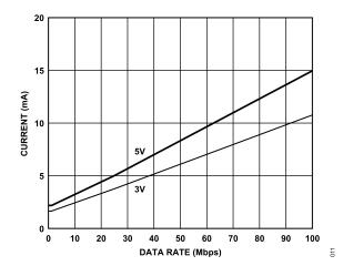
Figure 11. Typical ADuM2281 or ADuM2286  $V_{\rm DD1}$  or  $V_{\rm DD2}$  Supply Current vs. Data Rate for 5 V and 3 V Operation
