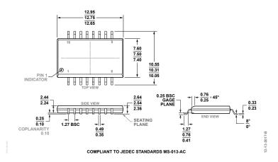
Figure 19. 16-Lead Standard Small Outline Package, with Increased Creepage [SOIC\_IC]
