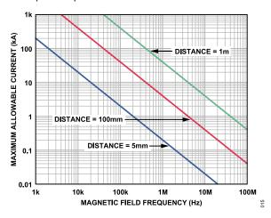
Figure 15. Maximum Allowable Current for Various Current to ADuM2280 Spacings
