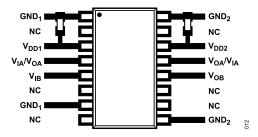
Figure 12. Recommended Printed Circuit Board Layout
