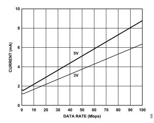
Figure 8. Typical Supply Current per Output Channel vs. Data Rate for 5 V and 3 V Operation (15 pF Output Load)
