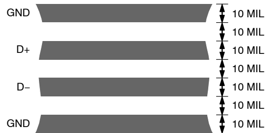
Figure 18. Arrangement of Signal Tracks
