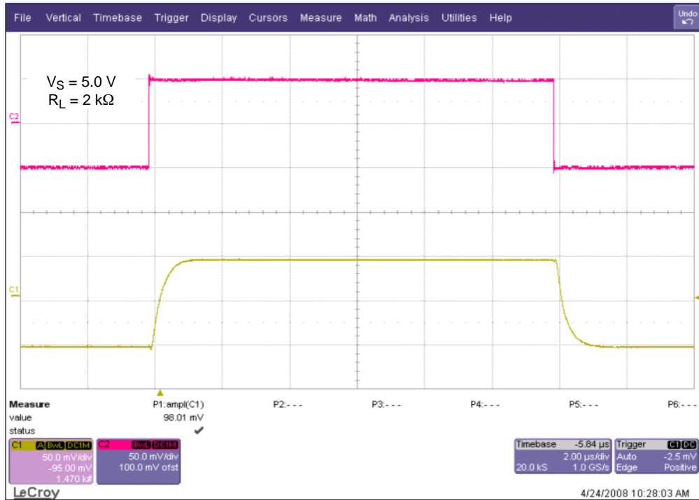
Figure 18. Small Signal Noninverting Response
