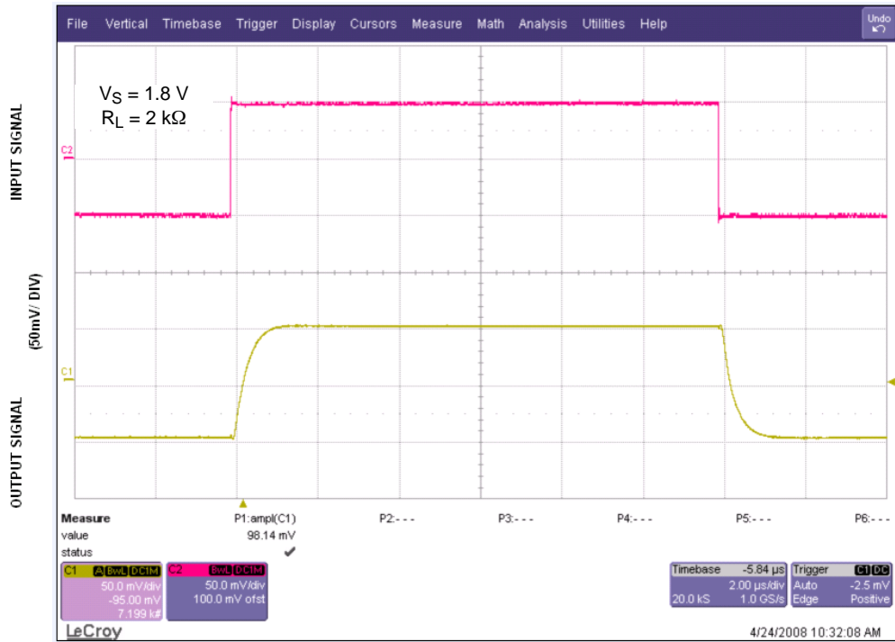
Figure 16. Small Signal Noninverting Response
