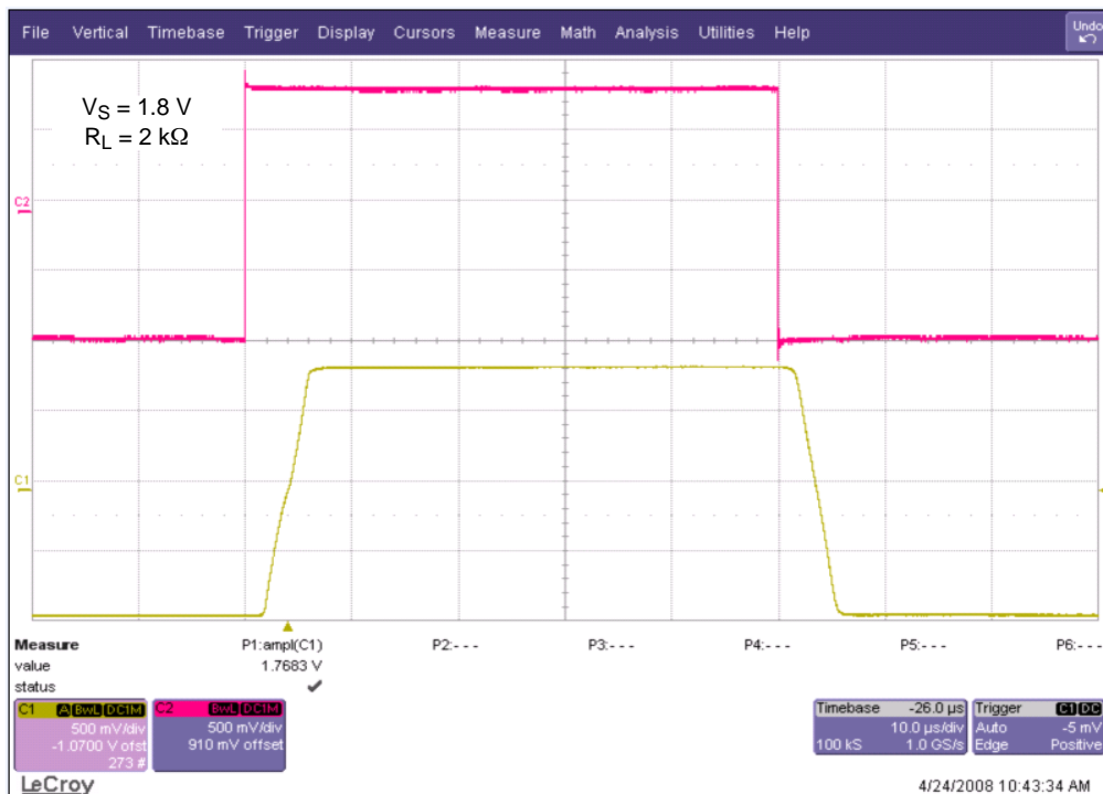
Figure 18. Small Signal Noninverting Response
