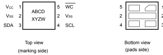
Figure 3. UDFPN5 (DFN5) package connections
