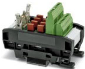
Varioface module intended for use with the ROC800 controller digital input cards
