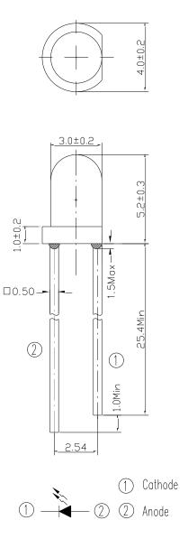
Note: Tolerances unless dimensions ±0.25mm
