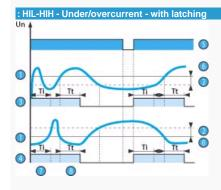
If "with memory" mode has been selected, the relay opens and stays in this position when threshold crossing is detected. The power supply must be disconnected to reset the product.
