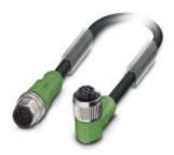
Sensor/actuator cable, 8-position, PUR halogen-free, black-gray RAL 7021, Plug straight M12, A-coded, on Socket angled M12, A-coded, cable length: 0.3 m
