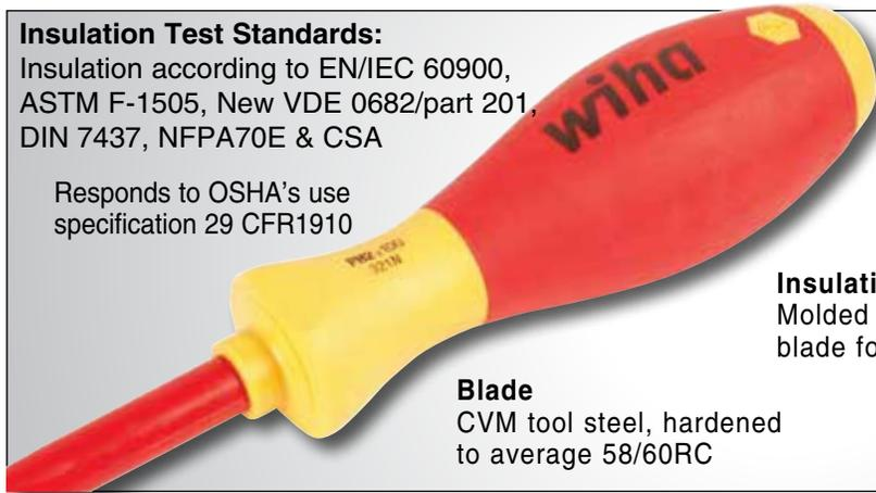
Each tool individually tested to 10,000 volts and rated to 1000 Volt ac or 1500 Volt dc
