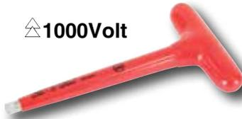
**29006 Insulated 1/4" Drive T-handle, With Insulated Handle.** Insulation according to EN/IEC 60900 & CSA specification, up to 1000 Volt. Individually Tested. Blade CV steel, hardened.
