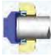
Installation Method B Thru Bore: Seal bottoms on machined bore shoulder
