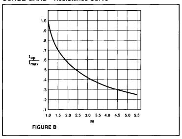
To determine the approximate resistance of a Ketema Rodan Surge-Gard operating at less than Imax, first determine the operating current ratio by dividing the actual operating current (Iop) by the respective Imax for the device being used.
