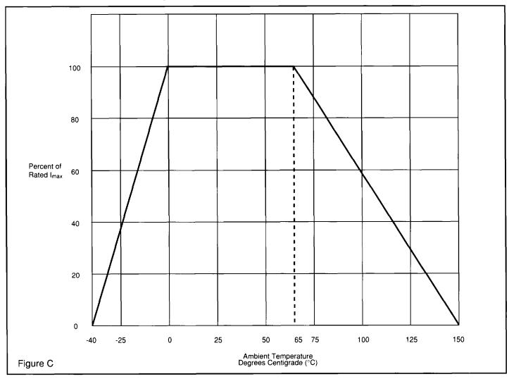
The recommended I<sub>max</sub> current versus the ambient temperature is shown in Figure C.
